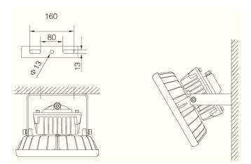
The model has a bracket/frame, the height of the whole lamp (includes the frame/ bracket) is 250mm).
